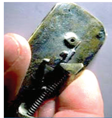
Fig 2 - Simple microscope created by Leeuwenhoek
